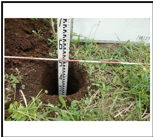
No.1掘削後GL-0.5m
